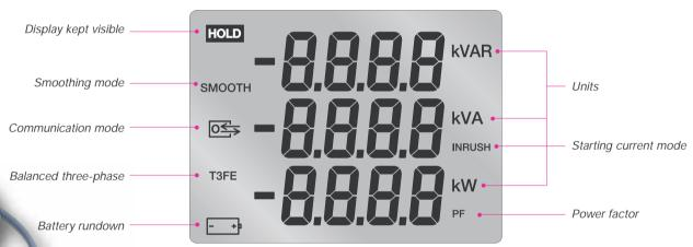
With the 73 x 54.3 mm LCD display, the user knows what the situation is at a glance. The battery rundown indicator light warns him when the period of autonomy is down to one hour.
