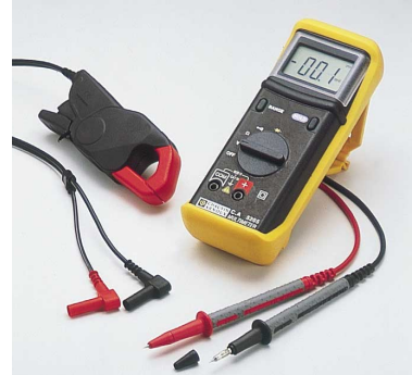
The C.A 5205G + miniclamp MN 89 set: measurement from 0.5 A to 240 A AC in complete simplicity and safety. Output/input ratio of the miniclamp: 100 mV DC/1 A AC.
