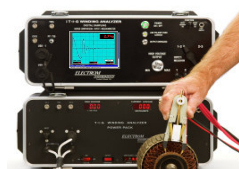
iTIG and Power Pack with Armature Test Fixture. ATF can be used for large and small armatures.
