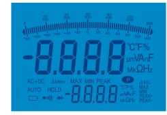
The large double LCD display with blue backlighting also offers a 61+2-segment full-scale bargraph. The Central Zero function allows you to view variations immediately. This type of bargraph is particularly practical for making adjustments.
