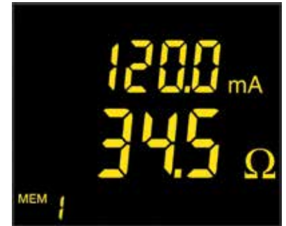
Standard mode: Impedance and leakage current
