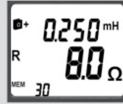
Screen 3: Value of the resistive and inductive part of the impedance measured
