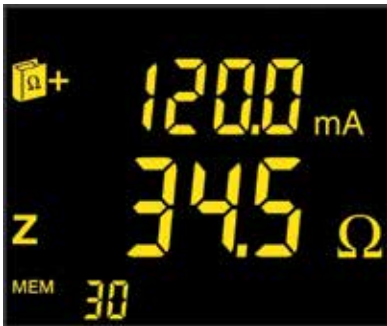
Screen 1: Impedance and leakage current
