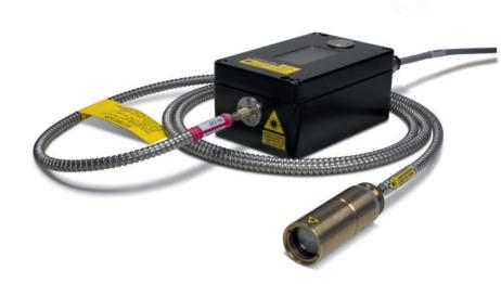
The pyrometers IS 50-LO plus and IGA 50-LO plus are digital, highly accurate infrared measuring instruments with fiber optics for non-contact temperature measurement on metals, ceramics, graphite etc. between 250 and 3500 °C.
