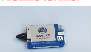
Trek's Model 950 Nozzle Ionizer provides fast and efficient removal of dust and static charge to help support manufacturing operations requiring a clean room environment. The compact ionizer uses high-pressure air flow to neutralize the static charge. It has a built-in high voltage power supply and an abnormal operation detection/warning function. The 950 operates by connecting a compressed air supply and a 24V power supply to the nozzle unit.
