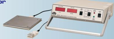
The Model 156A tests the efficiency of an ionizer's ion production by timing how long it takes air ions produced to discharge a floating plate that has been pre-charged to either a positive or negative value. The Model 156A also tests the balance between positive and negative air ions by measuring the offset voltage generated on a floating plate due to an imbalance of positive and negative air ions impinging on the plate from the ionizer.
