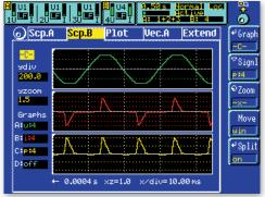
Scope function for waveform of sampling values
