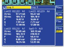
Calculation of the real values in the delta connected winding phases (wiring: 3+1,  $U\Delta$   $I* -> U\Delta$   $I\Delta$ )
