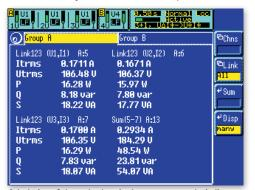
Calculation of the real values in the star connected winding phases (wiring: 3+1, U $\Delta$  I\* -> U\* I\*)
