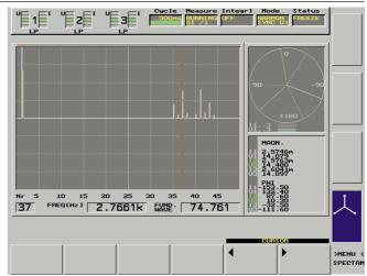
In the same way the shown phasor diagram belongs to the 37th. This frequency spectrum shows a very good suppression of the harmonics in the lower frequency range.
