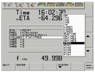
Using the integrated **formula editor** the user can build new values (VARiables) from all measured and computed values
