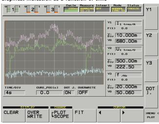
On pressing the 'Graph' key, the LMG310 switches to graphical display, showing the signals as a function of the time. The softkey 'PLOT/SCOPE'
