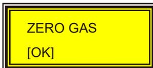
▲ Caution: Zero calibration should be processed with clean air or 99% nitrogen gas. (For O<sub>2</sub> gas, you must use nitrogen gas 99.8% or more.)
