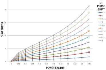
For example, with an uncorrected  $3^{\circ}$  phase angle error and reported power factor of 0.5, there is a corresponding kW error of >10%.
