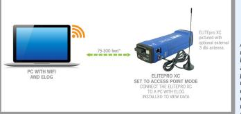
Access Point mode sets the ELITEpro XC as an access point. View real-time data on a wi-fienabled laptop running ELOG software
